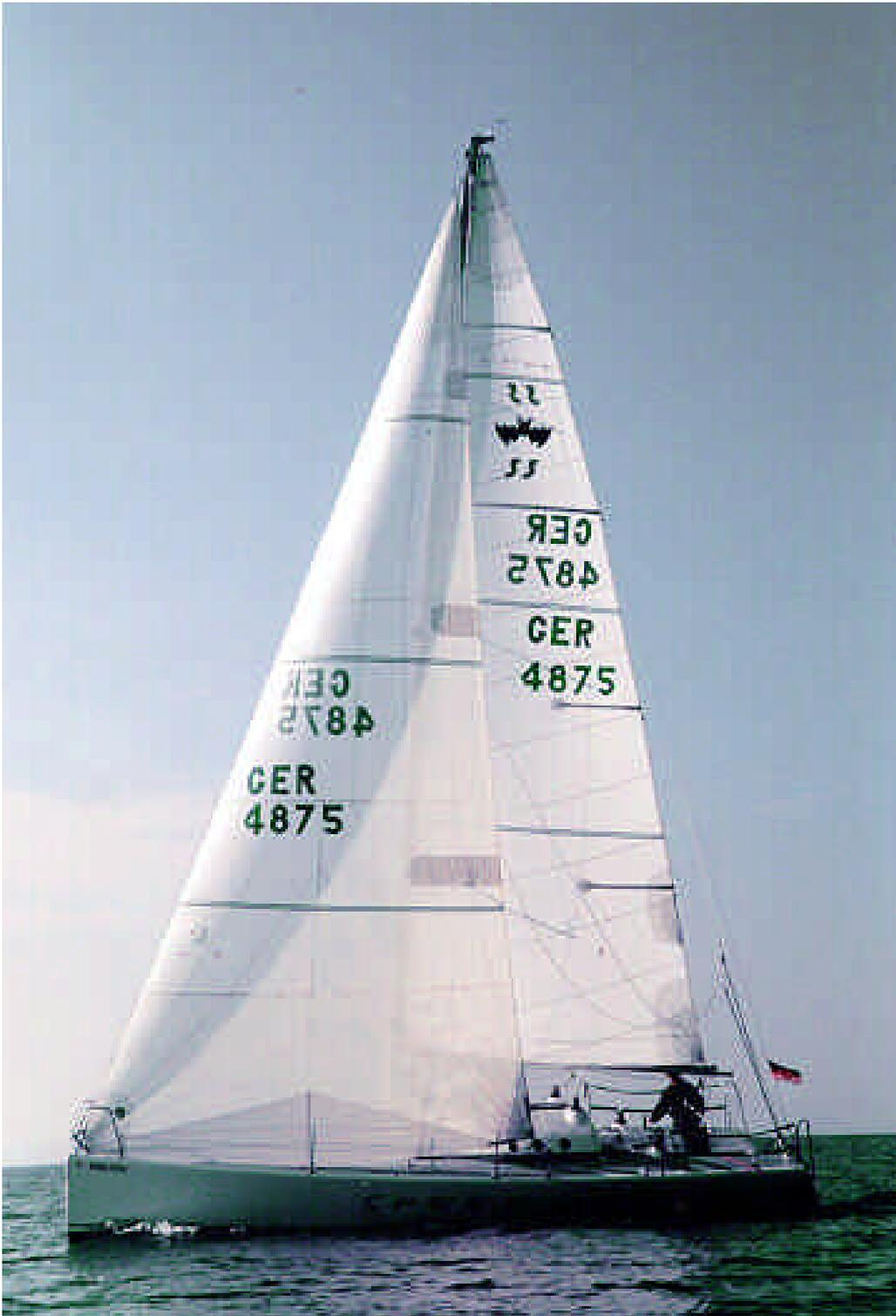
The ROMMEL 33 will carry a masthead rig with a maximum of 67 m<sup>2</sup> upwind. The light displacement of approx. 2.7 tons, the extremely slender hull and the enormous draught of 2.50 m provide her with optimal upwind performance. The 140 % genoa could be used when tacking at up to 15 knots. With the aid of a power-operated backstay, the mast profile can be set just as efficiently as with a 7/8 rig.
