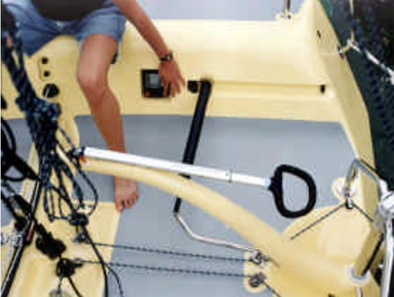
The position of the rudder is dependent on the draught - the optional autopilot is in idle position integrated in the cockpit wall.
