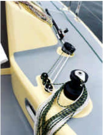
All cleaned up and ready for use: the control lines are guided under the genoa rail and the genoa barber, so that both genoa winches can be used.
