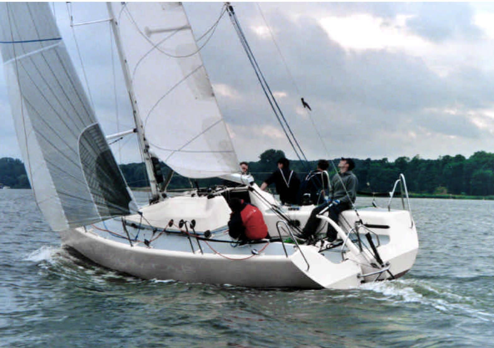
The lines of the ROMMEL 33 are characteristically very slender, with an extremely long waterline and a slightly concave transom.
