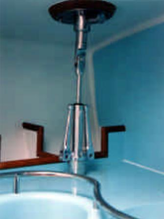
the rod rig can easily be eased and tensioned.
